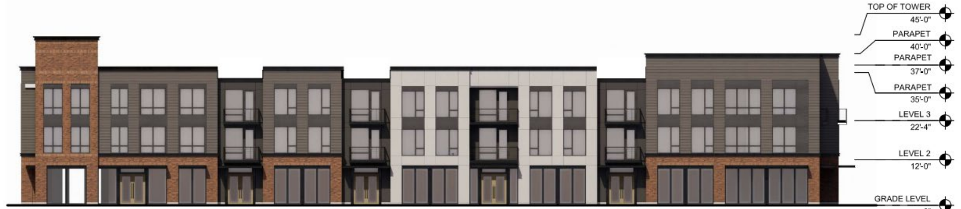
BUILDING 1 - NORTH ELEVATION
