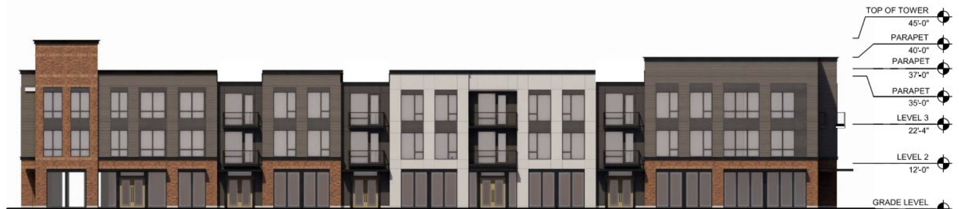
BUILDING 1 - NORTH ELEVATION
