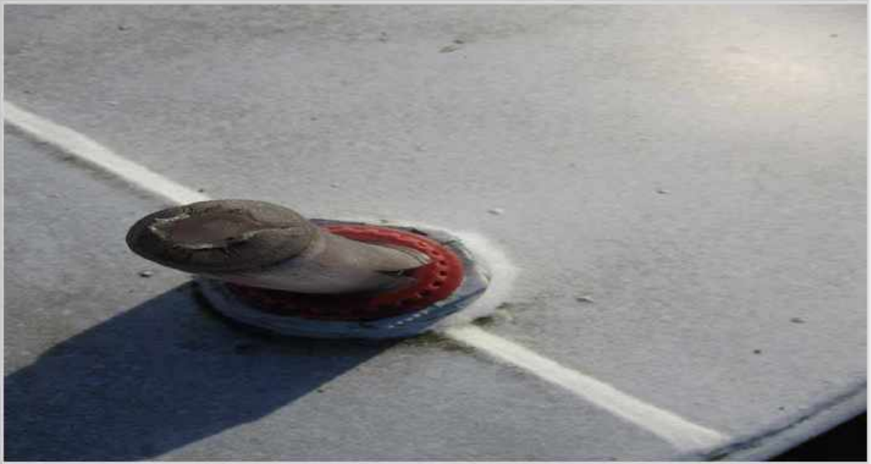
Exhibit "D" Damaged Mechanical Leak Detector
