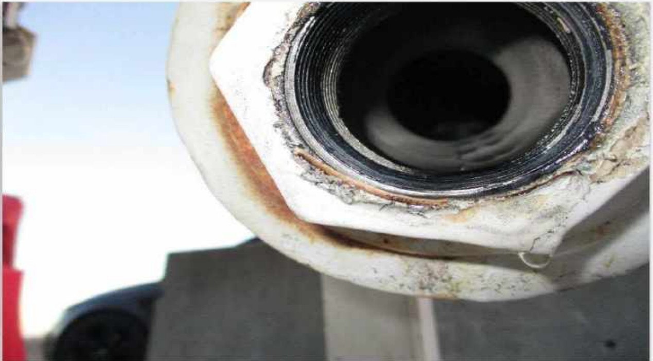
Exhibit "D" Damaged Mechanical Leak Detector
