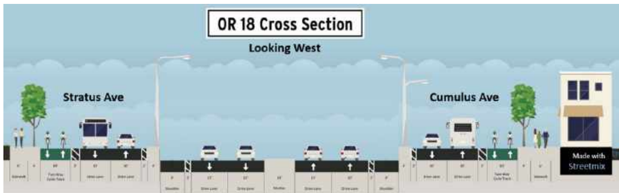
Figure 15. Proposed OR 18 Cross Section
