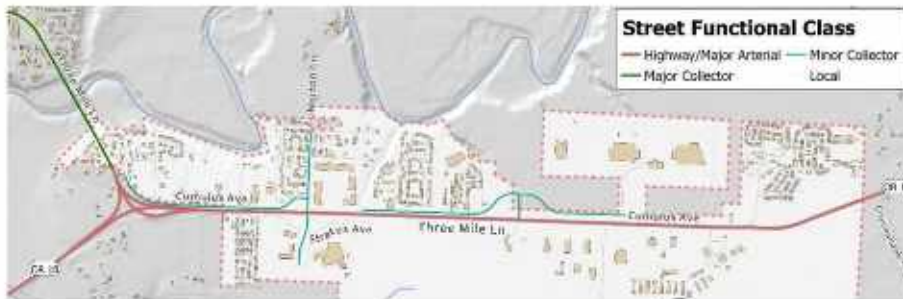
Figure 4. Street Network Functional Classification
