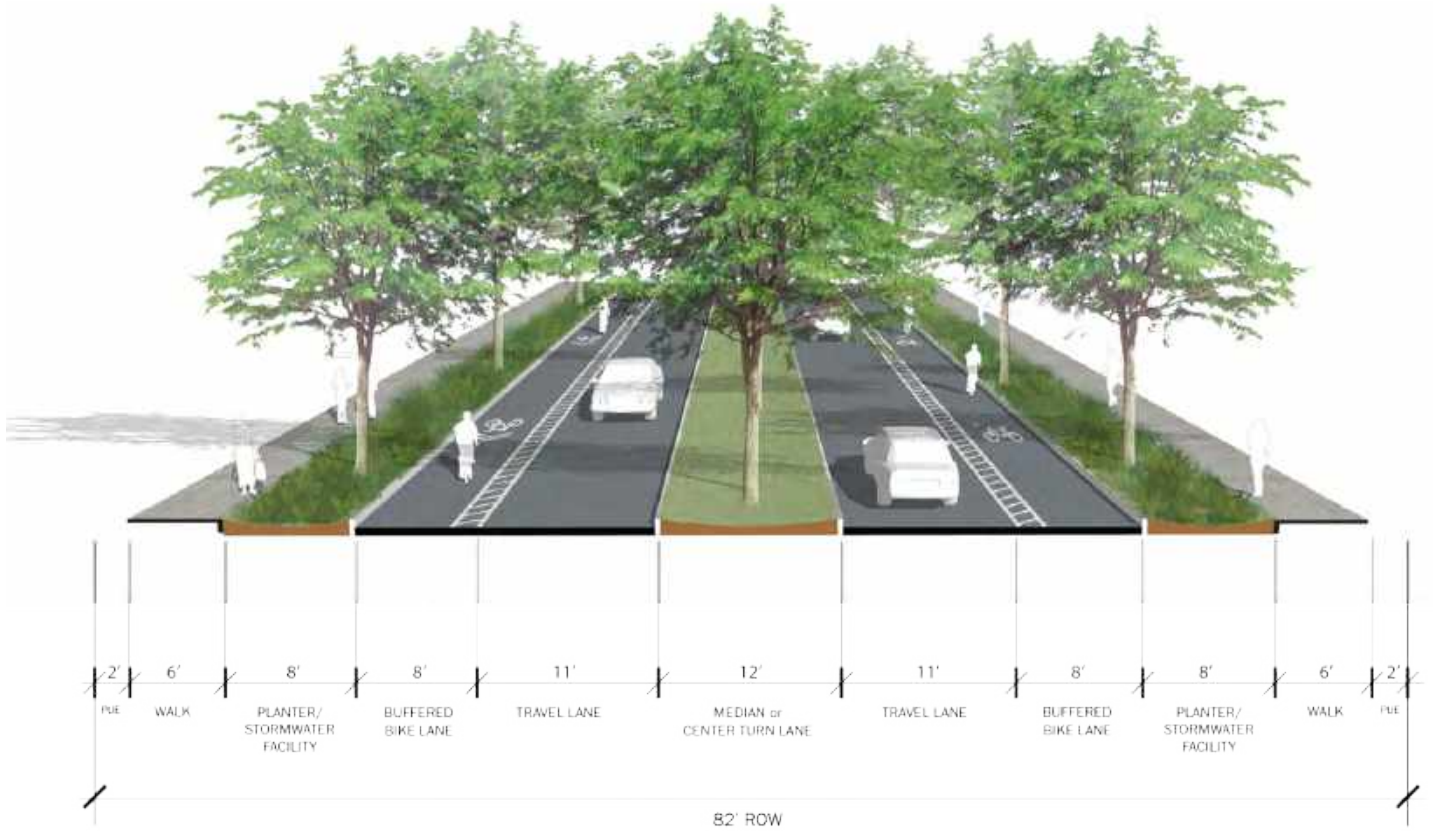
PROPOSED 3ML MAJOR COLLECTOR STREET CROSS-SECTION
