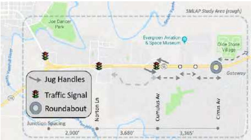
The Jug Handle concept removes all turn movements from the major highway and shifts them to the cross-street via a right-turn lane.
