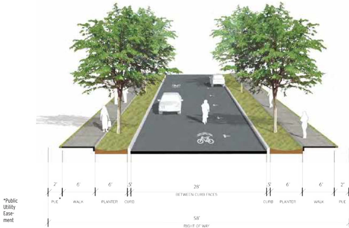
PROPOSED 3ML LOCAL RESIDENTIAL STREET CROSS-SECTION
