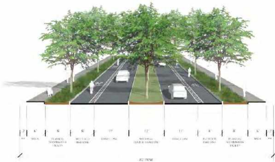
PROPOSED 3ML MAJOR COLLECTOR STREET CROSS-SECTION
