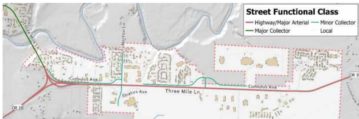
Figure 4. Street Network Functional Classification
