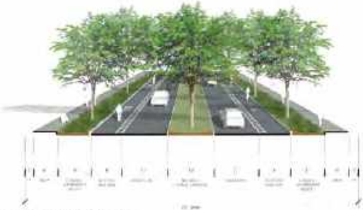
PROPOSED 3ML MAJOR COLLECTOR STREET CROSS-SECTION
