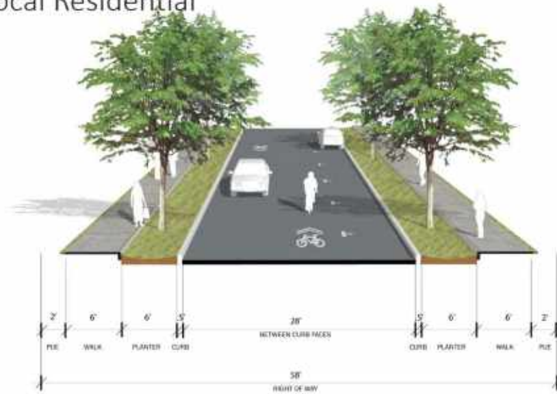
Figure 17. Local Residential Street Cross Section
