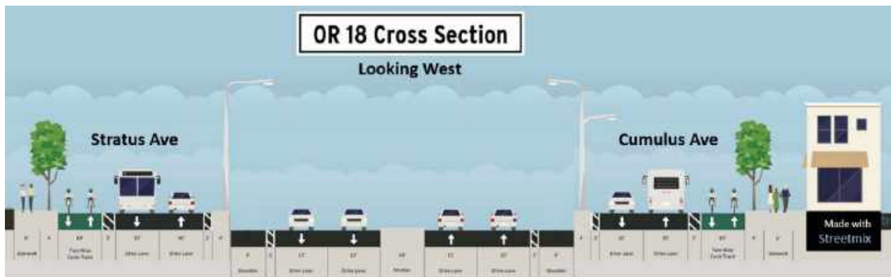
Figure 15. Proposed OR 18 Cross Section
