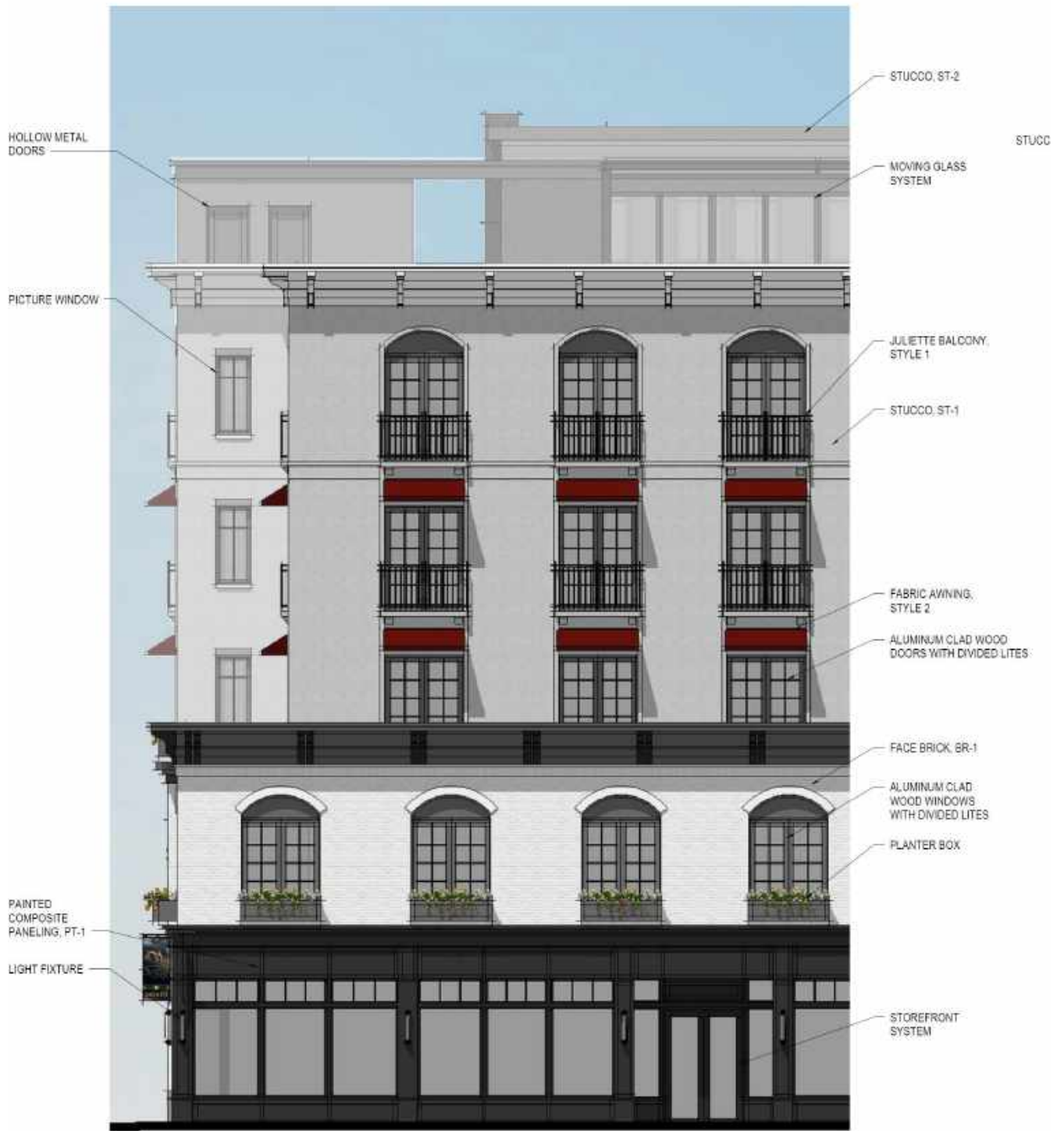
ENLARGED PARTIAL ELEVATION - 3RD STREET
