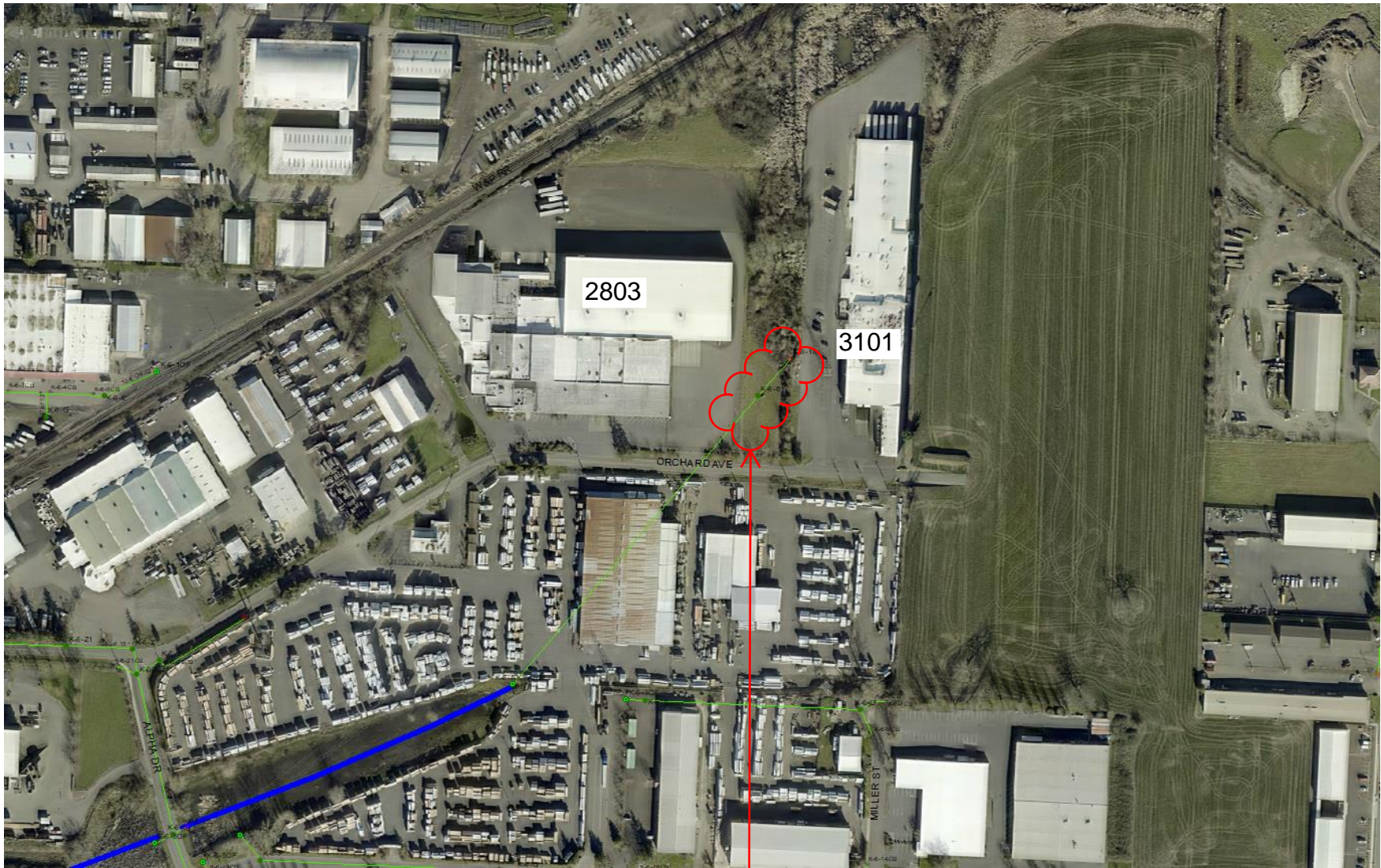
Area of failed corrugated metal storm main to be replaced.
