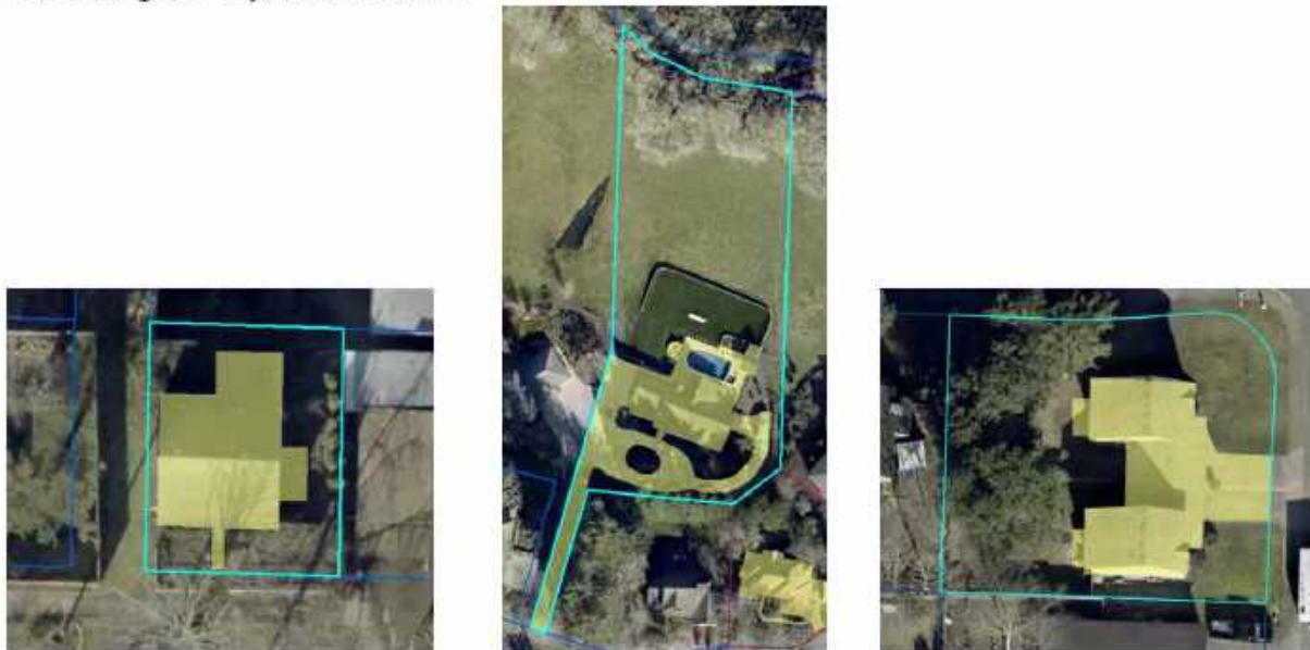
Figure 2. Example of SFR Properties’ Impervious Area Digitization (photos not at the same scale)
