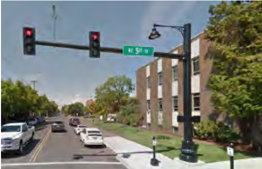
Where applicable, the historic pendant light fixtures will be affixed to signal poles with decorative bases (RIGHT). The LEFT image above shows a recently-installed example at NE 5th and Evans Streets in Downtown McMinnville.
