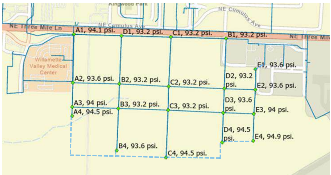
Figure 2-3. MDD Pressures. Recommended looping (dashed lines) improves water circulation and water quality.
