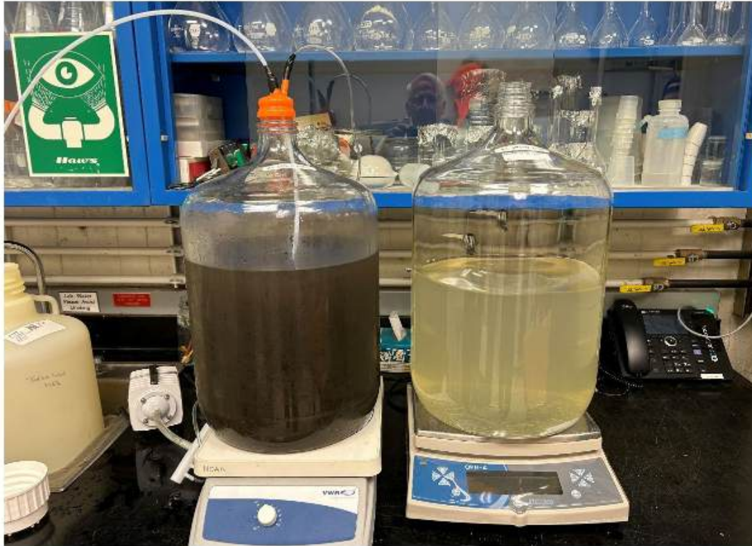
Figure 4. Sub-sampling apparatus using positive pressure and continuous stirring for homogenous sub-sampling.
