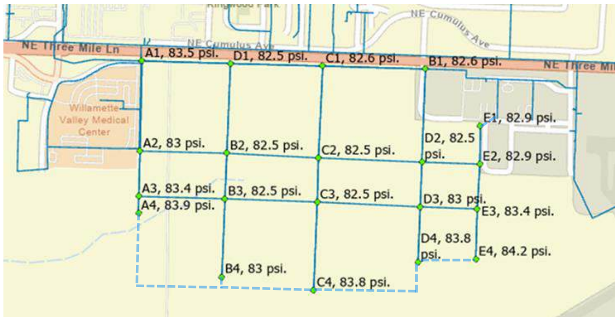
Figure 2-4. PHD Pressures. Recommended looping (dashed lines) improves water circulation and water quality.
