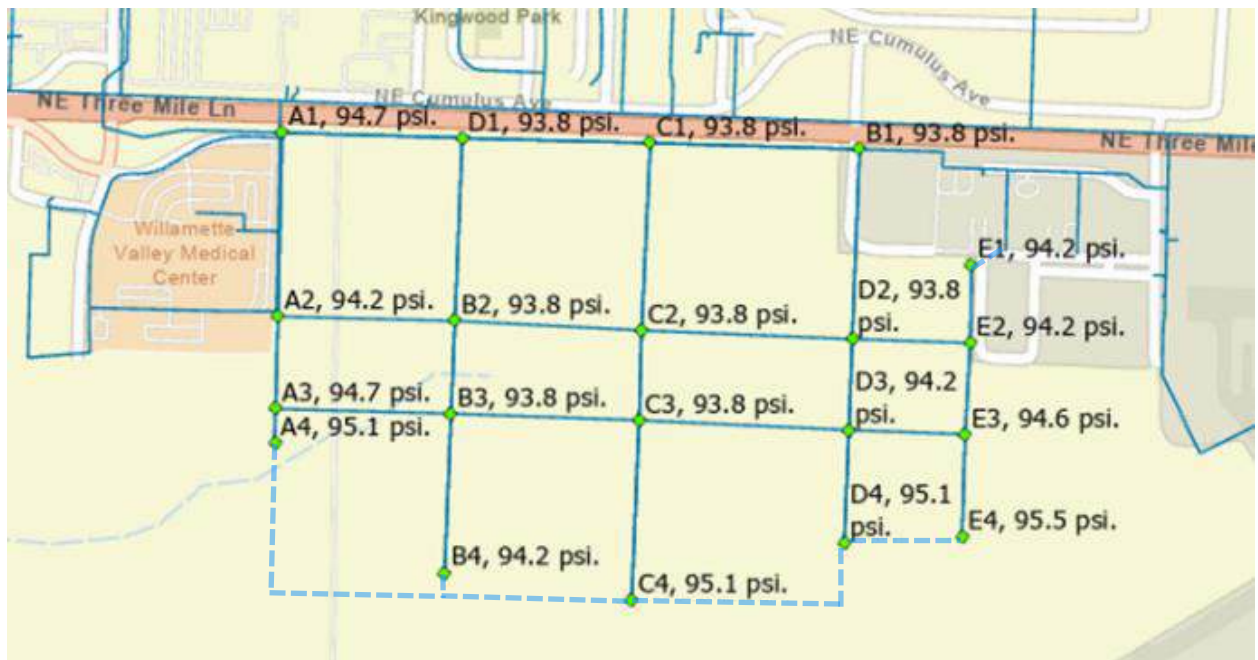
Figure 2-2. ADD Pressures. Recommended looping (dashed lines) improves water circulation and water quality.
