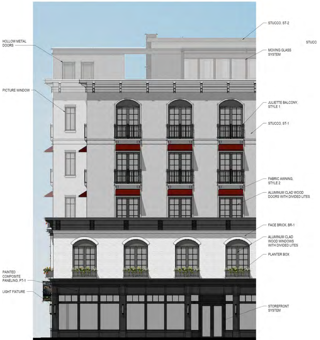
ENLARGED PARTIAL ELEVATION - 3RD STREET
