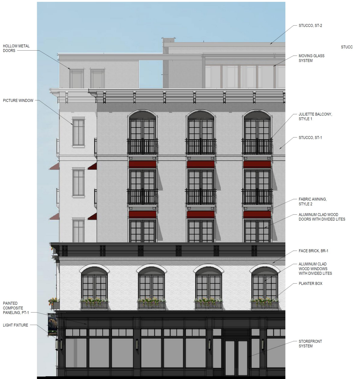
ENLARGED PARTIAL ELEVATION - 3RD STREET
