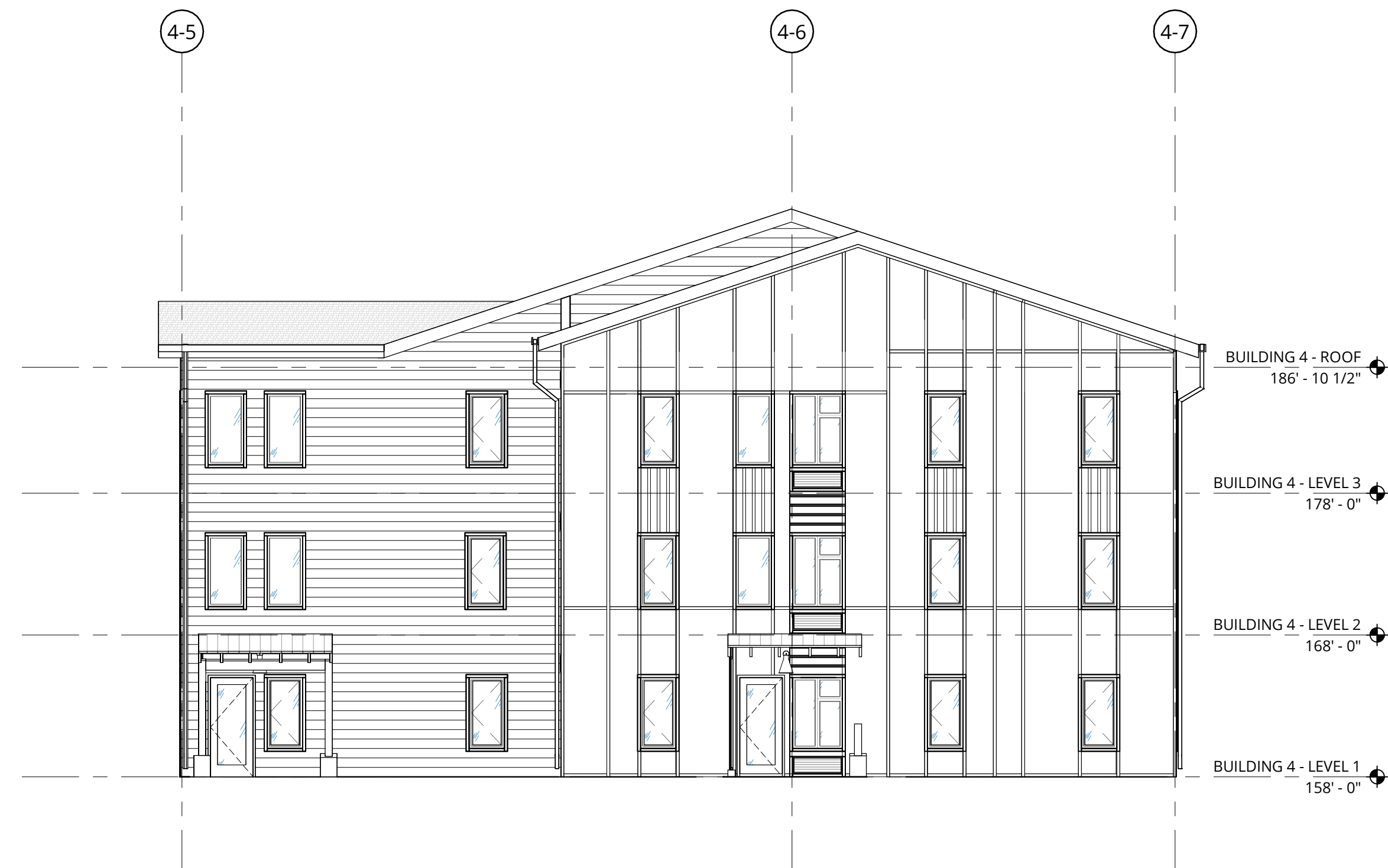
4 BUILDING 4 - WEST ELEVATION 2 1/8" = 1'-0"
