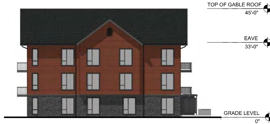
BUILDING 5 - EAST ELEVATION
