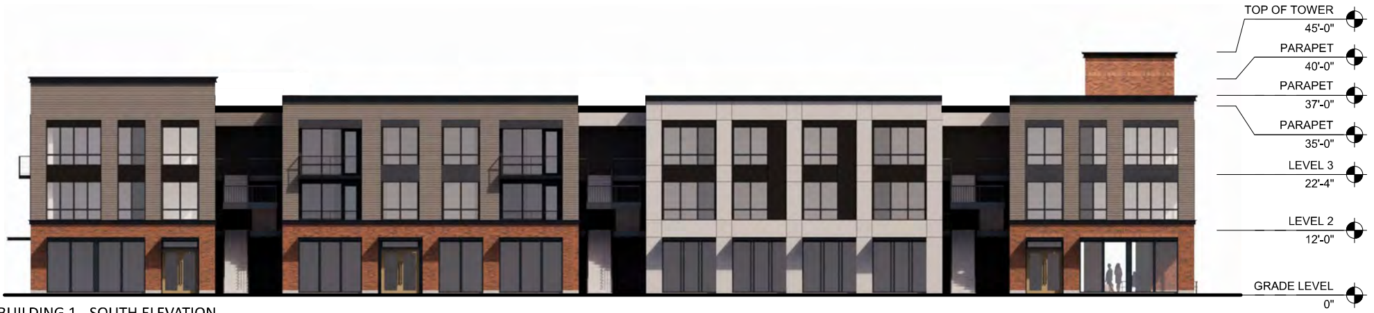
BUILDING 1 - SOUTH ELEVATION
