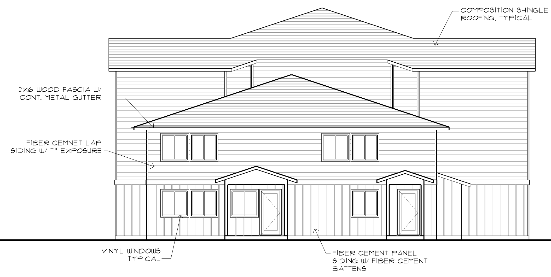
BUILDING 'B' - NORTH ELEVATION 3 Scale: 1/8" = 1'-0" A7.2
