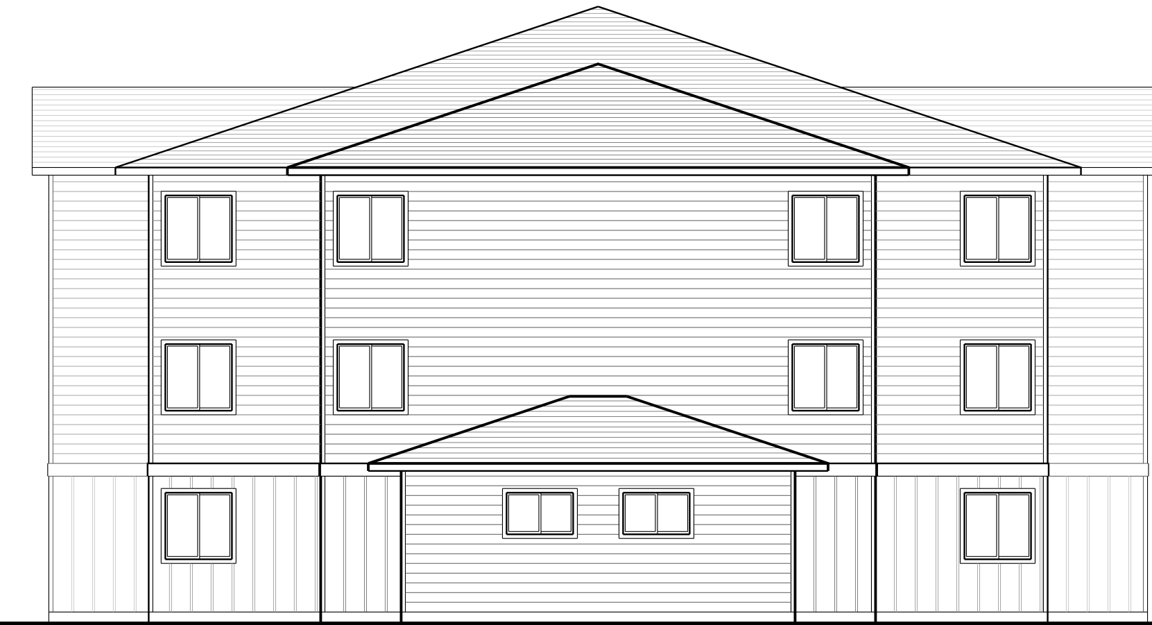
BUILDING 'E' - EAST ELEVATION 3 Scale: 1/8" = 1'-0" A7.5
