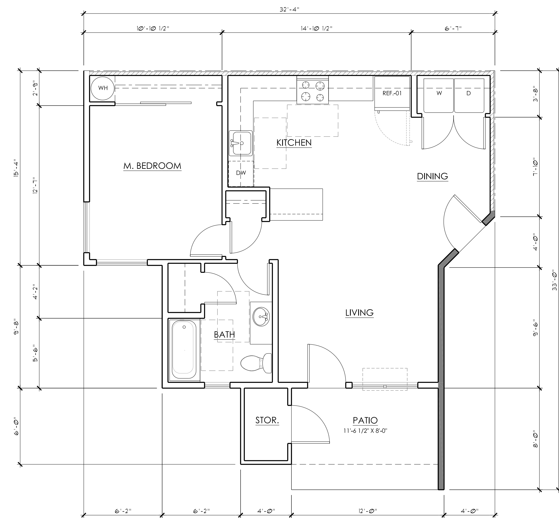
703 SF UNIT TYPE D-B, 1BR, 1 BATH, ADA TYPE 'B' END UNIT 3 Scale: 1/4" = 1'-0" A4.1
