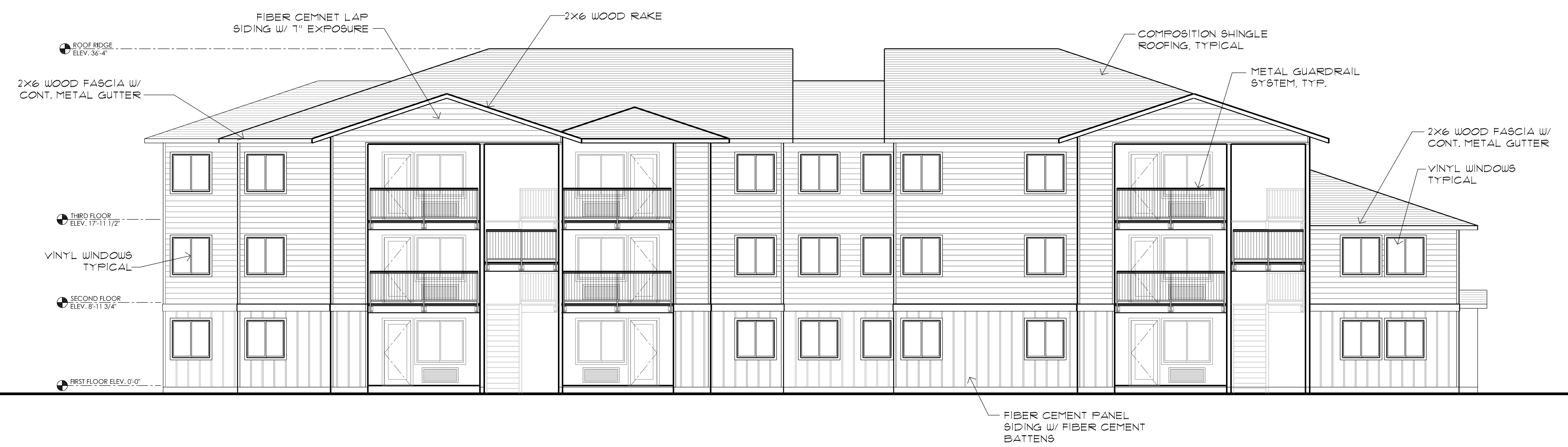
BUILDING 'B' - EAST ELEVATION 1 Scale: 1/8" = 1'-0" A7.2
