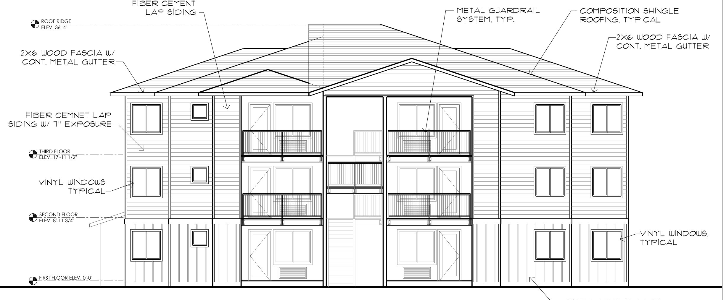
BUILDING 'A' - WEST ELEVATION 4 Scale: 1/8" = 1'-0" A7.1
