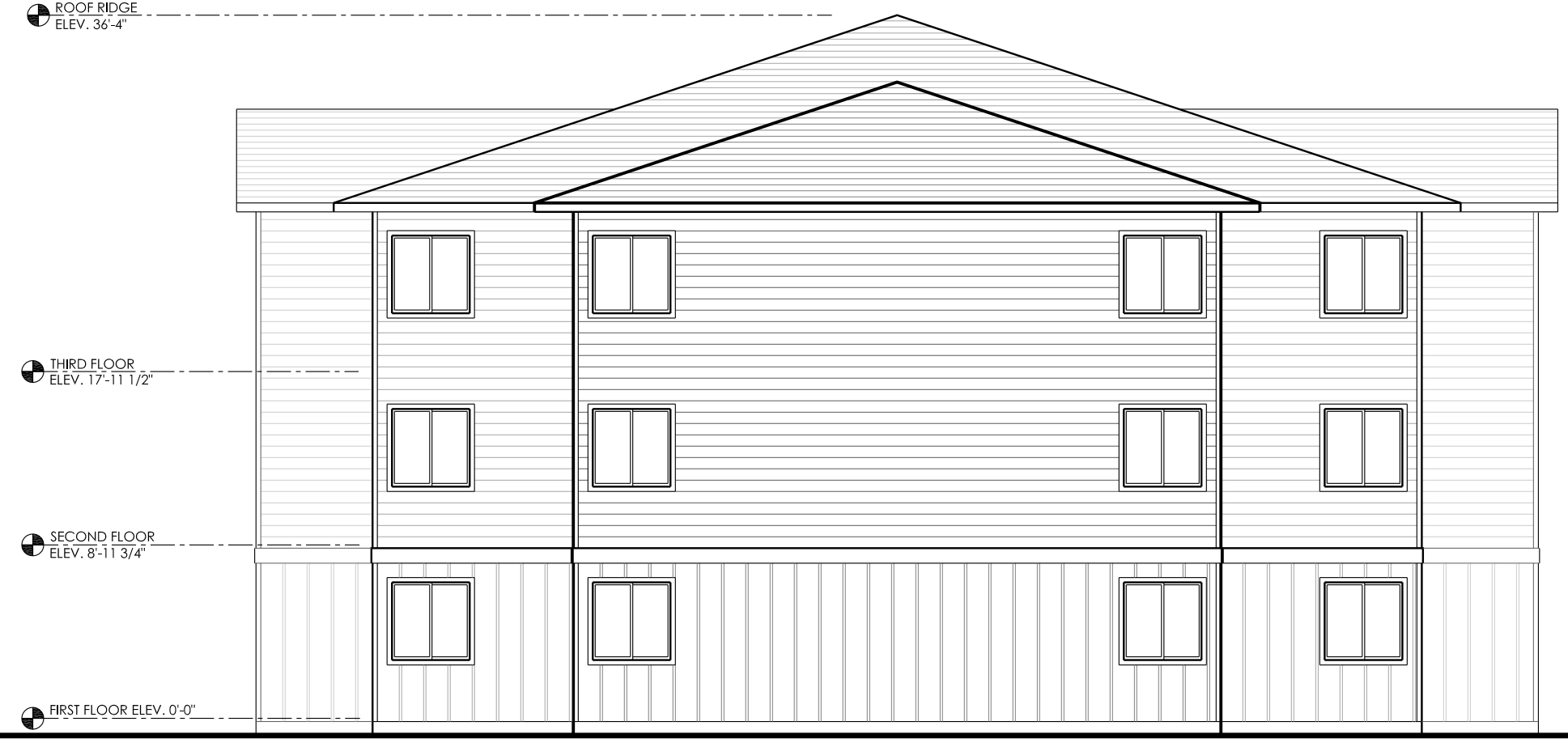
BUILDING 'G' - NORTH ELEVATION 3 Scale: 1/8" = 1'-0" A7.7
