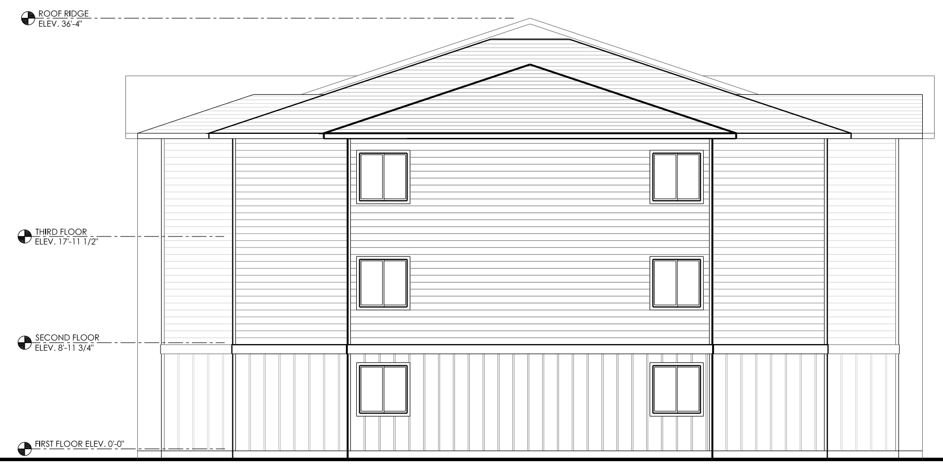
BUILDING 'D' - SOUTH ELEVATION 2 Scale: 1/8" = 1'-0" A7.4
