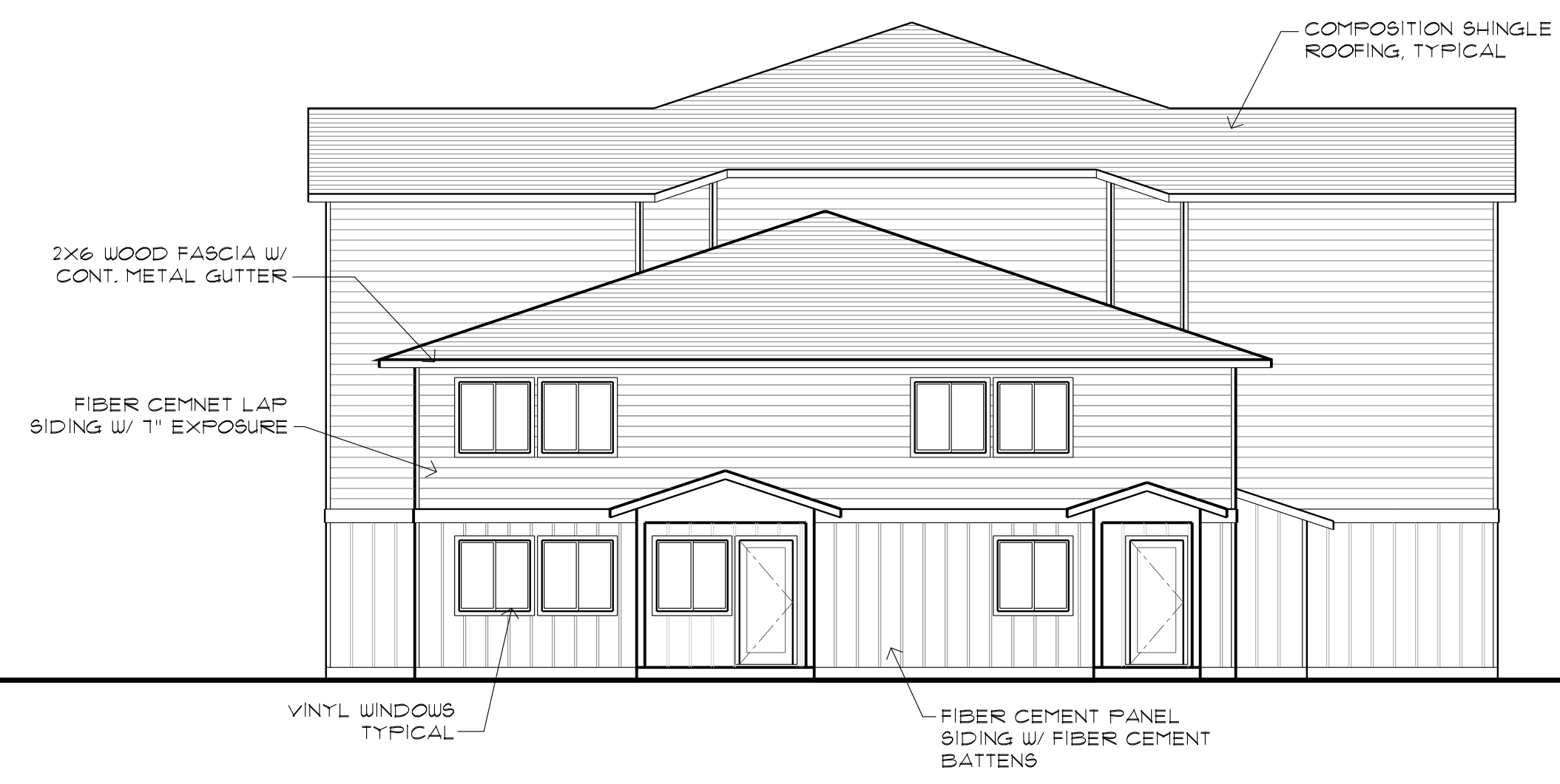
BUILDING 'B' - NORTH ELEVATION 3 Scale: 1/8" = 1'-0" A7.2
