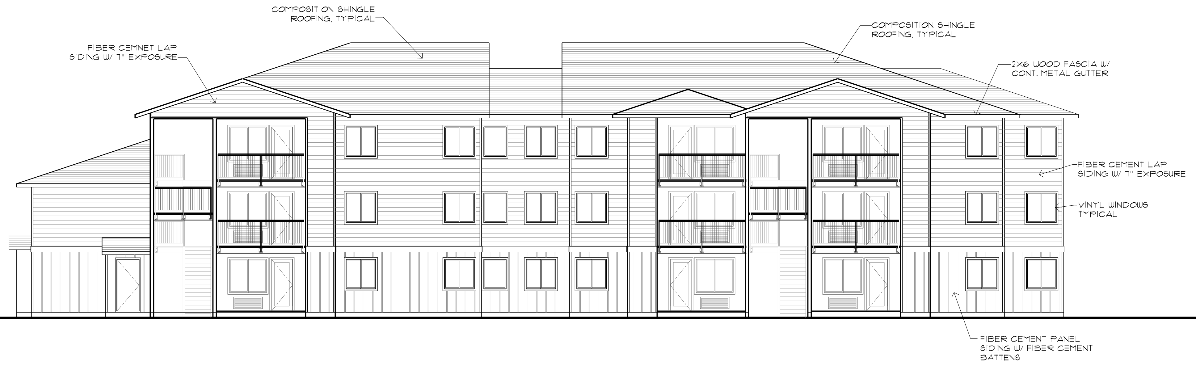
BUILDING 'B' - WEST ELEVATION 4 Scale: 1/8" = 1'-0" A7.2
