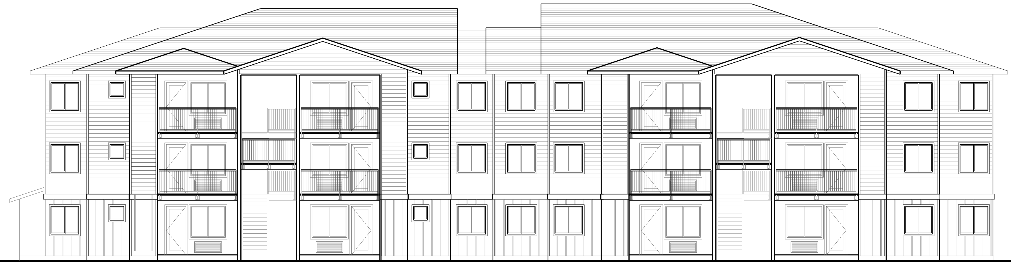
BUILDING 'G' - EAST ELEVATION 1 Scale: 1/8" = 1'-0" A7.7
