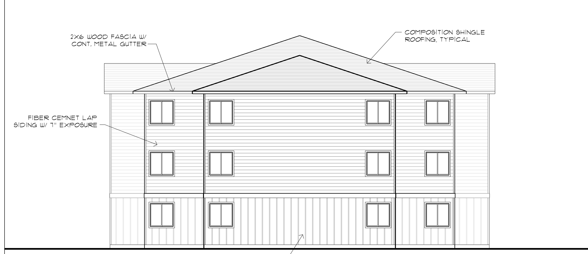
BUILDING 'A' - NORTH ELEVATION 3 Scale: 1/8" = 1'-0" A7.1
