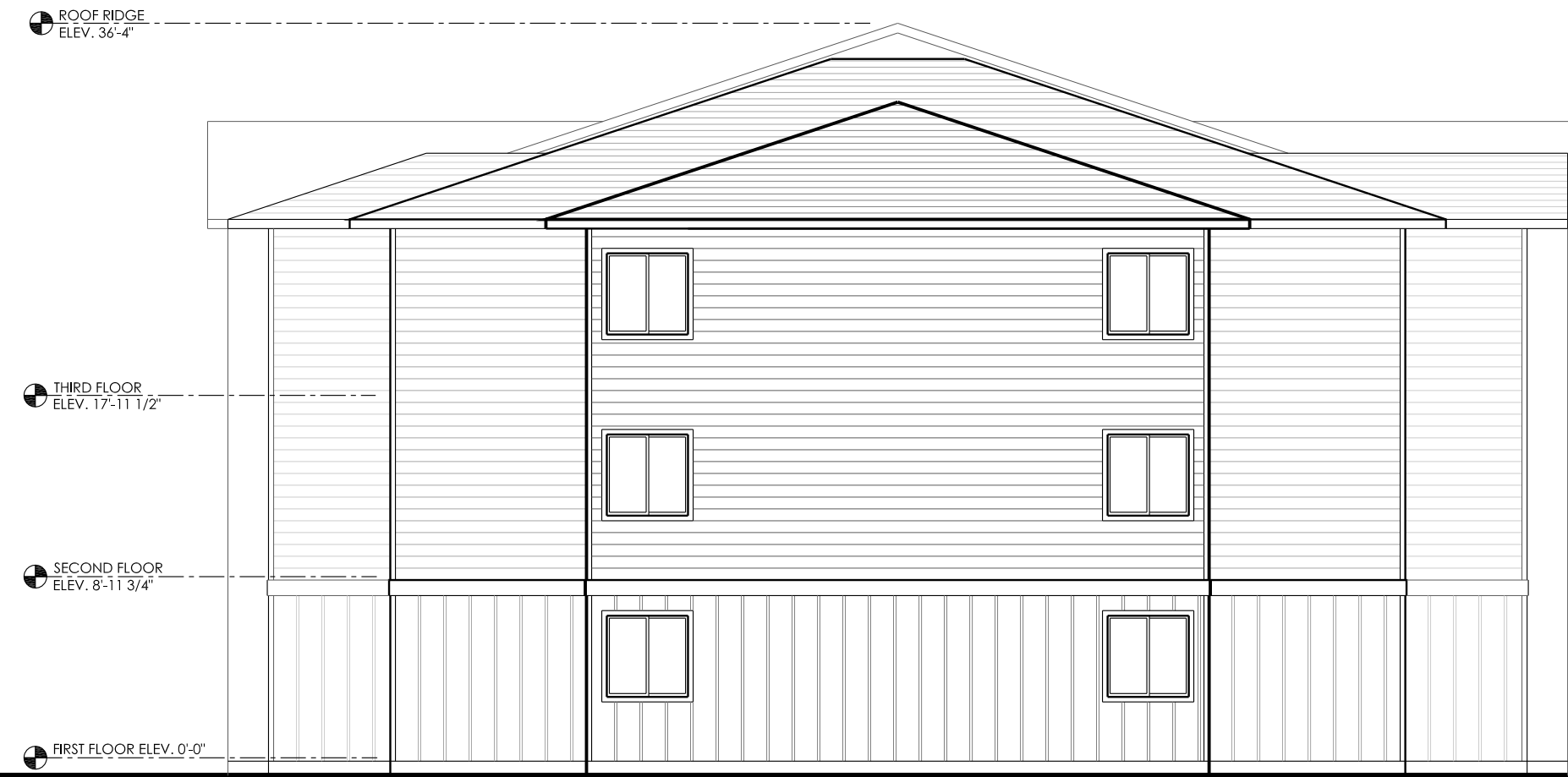
BUILDING 'E' - WEST ELEVATION 2 Scale: 1/8" = 1'-0" A7.5
