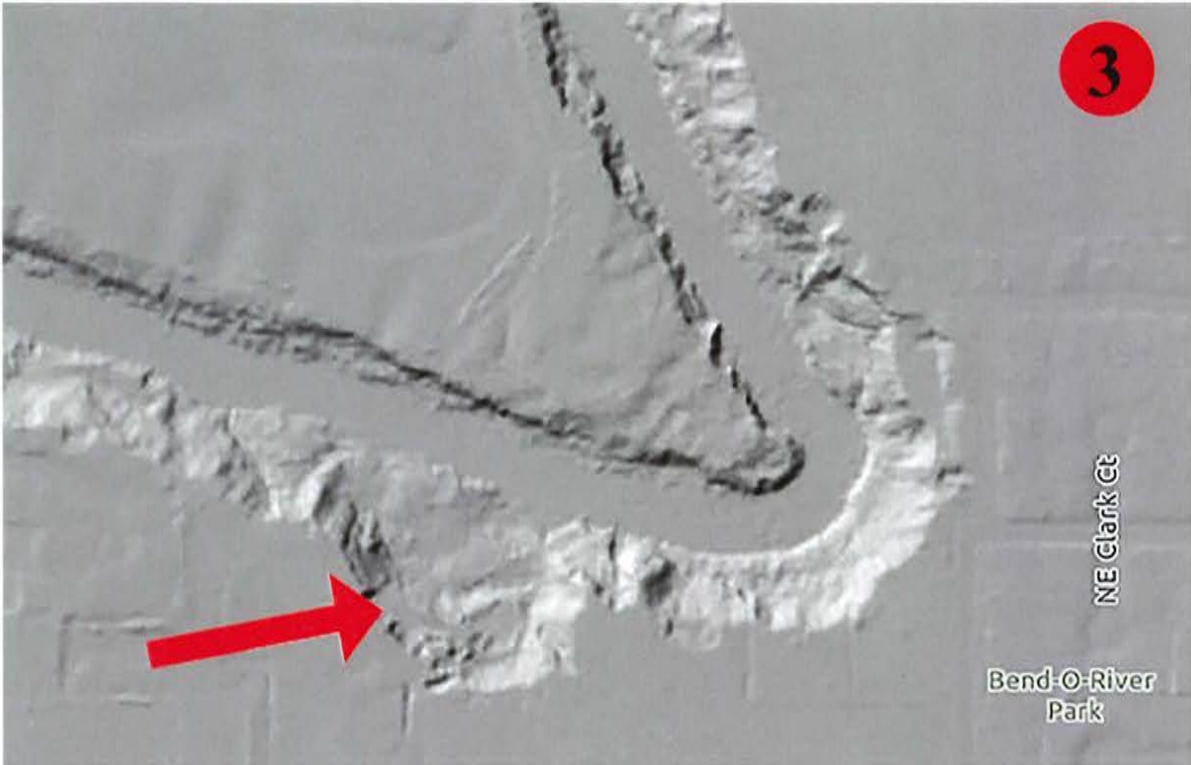
A mass wasting block just upstream from the proposed development (highlighted below) borders a concrete plant.
