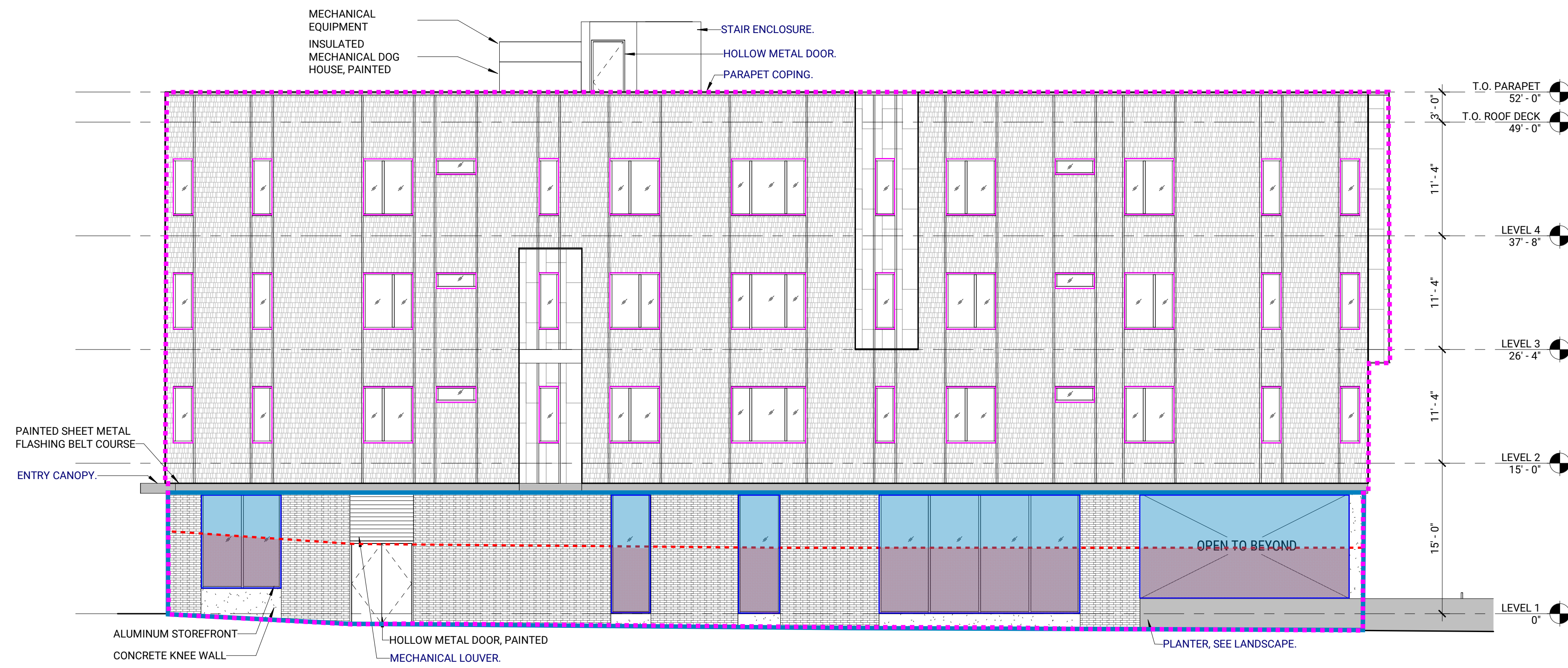
C1 EXTERIOR ELEVATION - WEST 1/8" = 1'-0"
