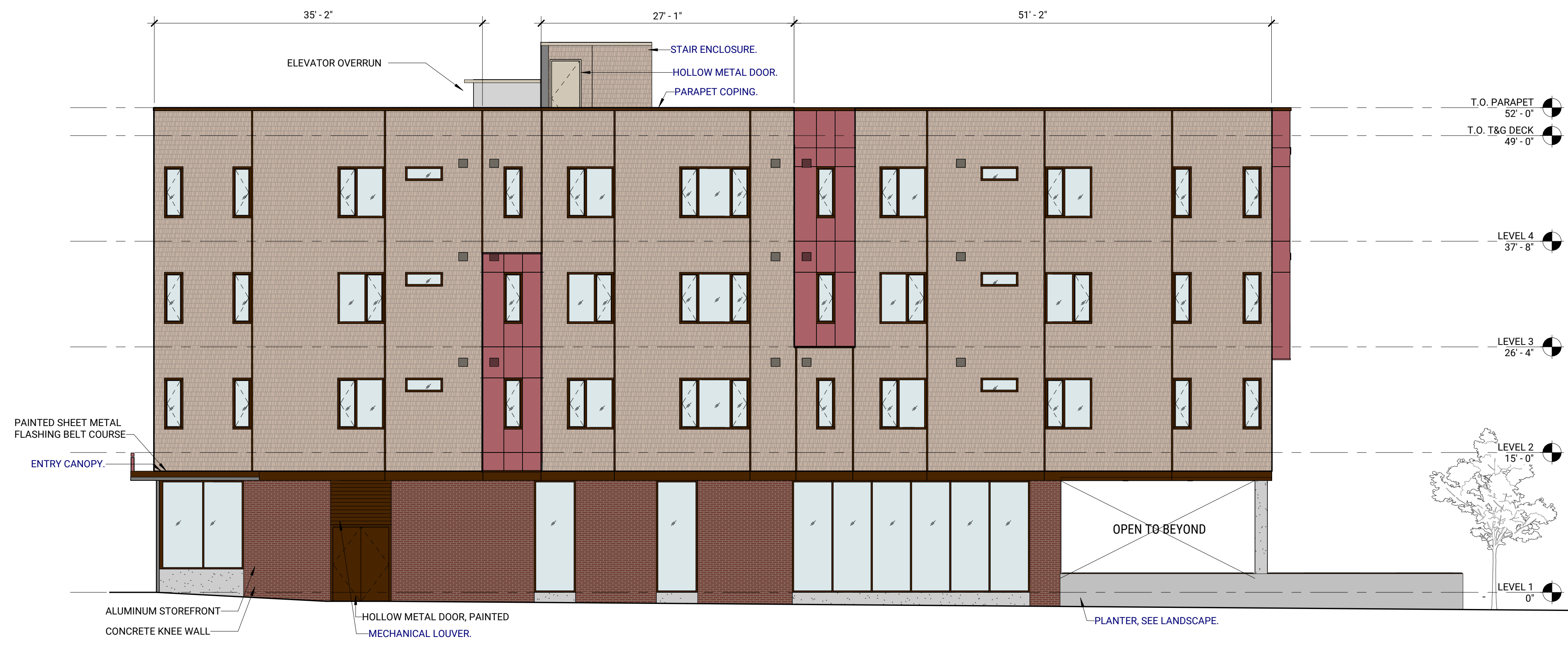
C1 EXTERIOR ELEVATION - WEST 1/8" = 1'-0"
