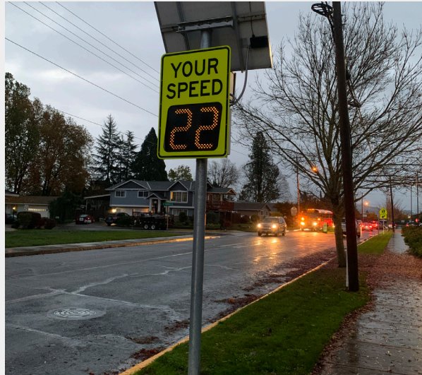
Radar speed feedback signage along Davis St lets cars know if they're exceeding the speed limit as they pass the school campus.
