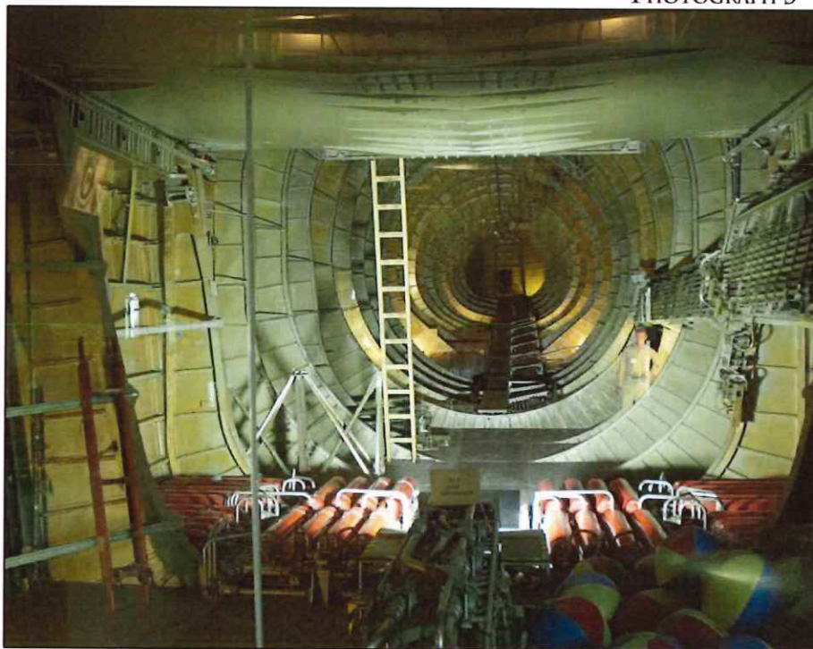
THE H-4 HERCULES CARGO DECK, LOOKING AFT FROM THE VIEWING CUBE TOWARD THE SEAPLANE'S TAIL. THE WINGS COME TOGETHER AT TOP OF THE IMAGE, ACCESSIBLE BY THE LADDER AT THE CENTER. THE RESTORATION CREW DISCOVERED THE BEACH BALLS (LOWER RIGHT) IN THE PONTOONS. NOTE THE RED CO 2 CANISTERS, WHICH ARE PART OF THE FIRE SUPPRESSION SYSTEM.
