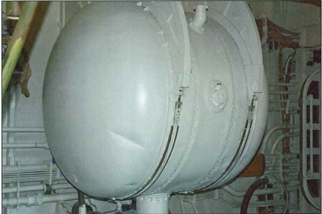
THE 281-GALLON OIL STORAGE TANK, SITS JUST OUTSIDE THE PORT SIDE LEADING EDGE WING ACCESS DOOR, AFT, ON THE H-4 HERCULES FLIGHT DECK.
