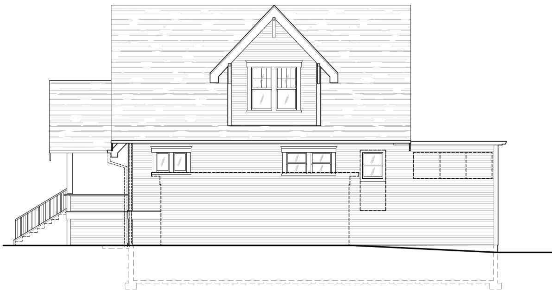
6 HISTORICAL HOUSE— MODIFIED EAST ELEVATION W/OUT GARAGE A1.5 SCALE: 3/16"=1'-0"
