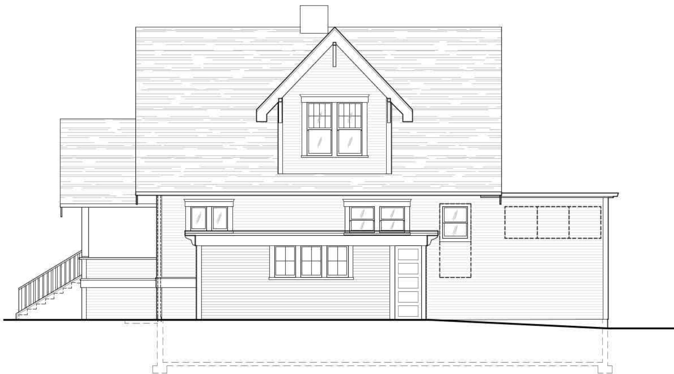
2 HISTORICAL HOUSE— MODIFIED EAST ELEVATION A1.5 SCALE: 3/16"=1'-0"
