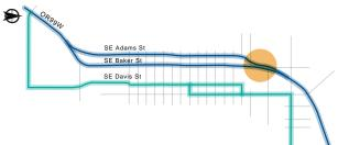
Construct median to prevent overlapping left-turns OR99W (Pacific Highway W) FIGURE
