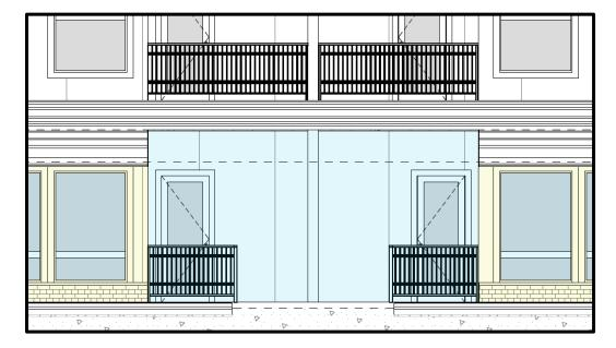
A condition of approval is required that the final construction plans be revised to include a more defined transom on the ground floor apartment unit entrances that open onto the NE 1<sup>st</sup> Street right-of-way.
