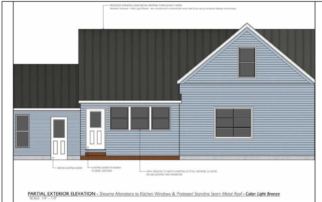
**Figure 3. Illustrations of Window Alteration**
