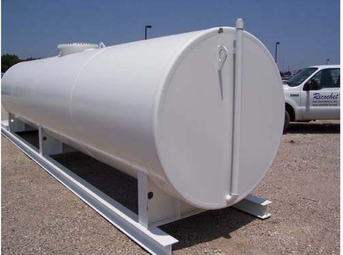
Photo No. 3: This is a photo of a 20,000 gallon fuel tank.
