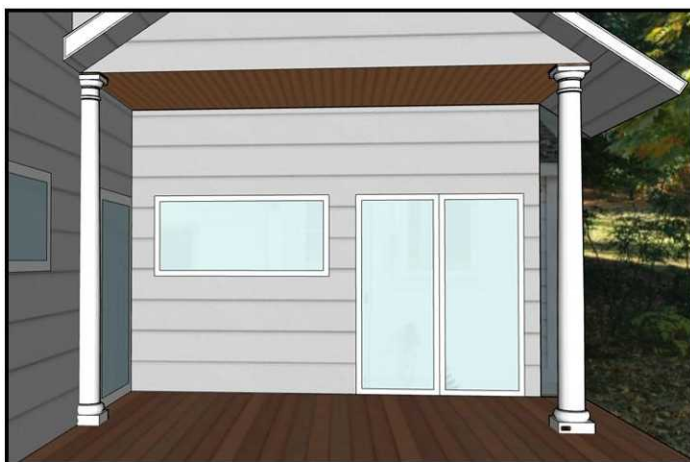
Figure 7: (Left) Proposed exterior of East side of home with porch additions removed. Note addition of extended roofline to accommodate sheltered walkway and columns to match those seen on front porch of home (right).
