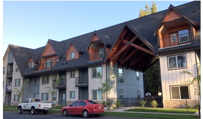
The use of roof forms and changes in materials and colors that reflect units of living decreases the perception of the massing and scale of this apartment building.
