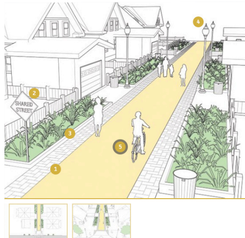
Showing an alley with a 28-foot right of way width and a 14-foot travel way (NACTO)
