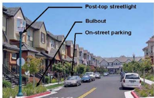
RECOMMENDED - Streets should include adequate space for street parking, sidewalks, and planting strips.
