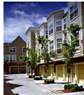
RECOMMENDED - An appropriately designed auto court with articulating upper stories that include bays, balconies, and modulating building mass reduces the "canyon" perception of a private street.
