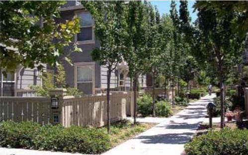
RECOMMENDED - Fencing should be designed to integrate into the architecture of the buildings and add visual interest in its detail, materials or color.
