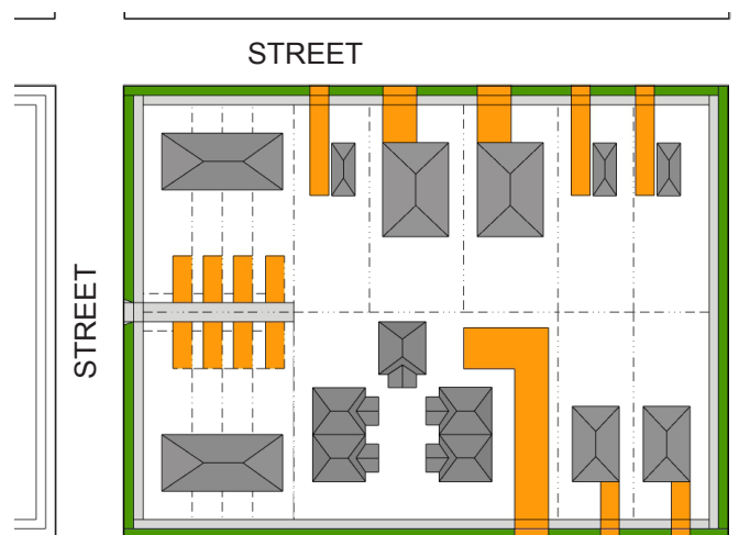
Hybrid infill block layout with partial alley at one end of a block and front-loaded parking for the remainder.
