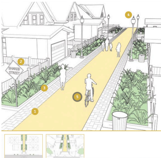
Showing an alley with a 28-foot right of way width and a 14-foot travel way (NACTO)
