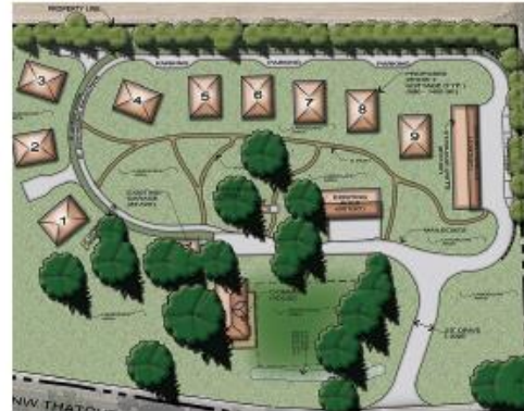
Cottage cluster design with shared common house and parking grouped in small areas.
