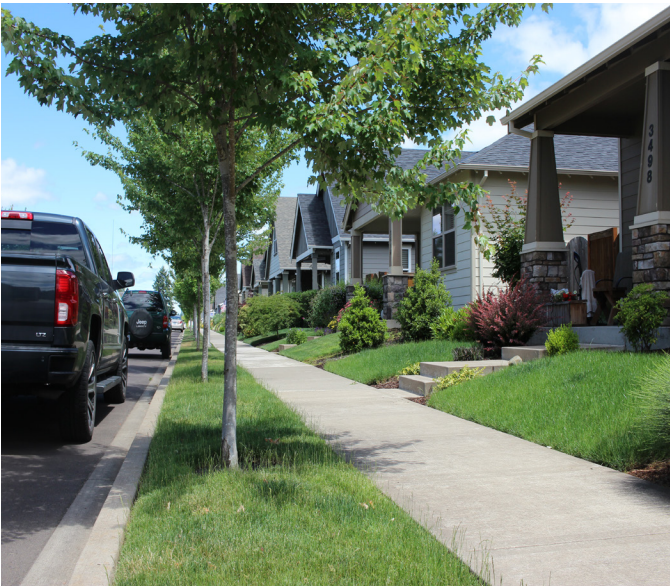
There is room for a continuous planter strip with ample street trees when parking is accessed from an alley.
