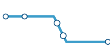
Inconsistent stop spacing
