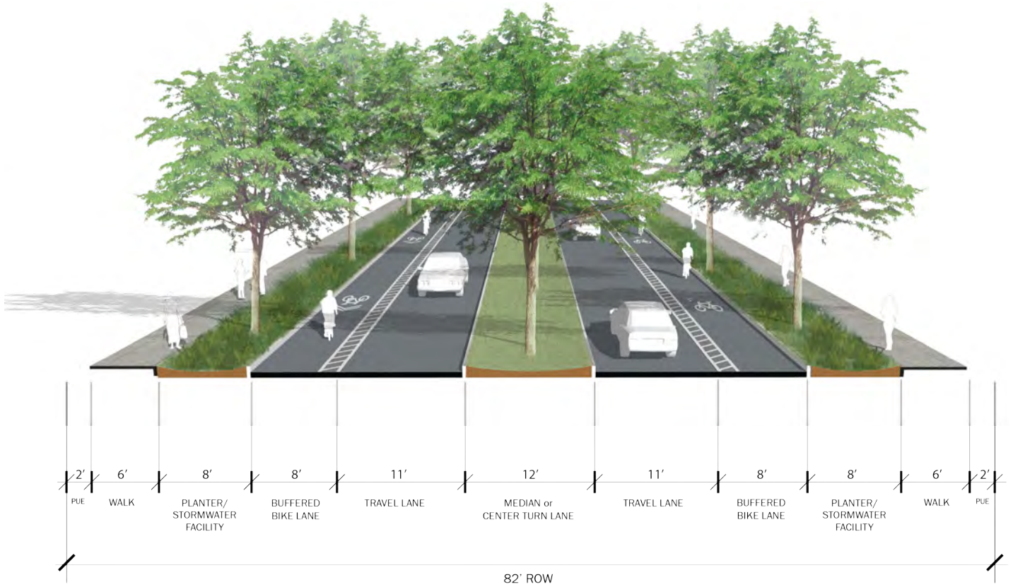
PROPOSED 3ML MAJOR COLLECTOR STREET CROSS-SECTION
