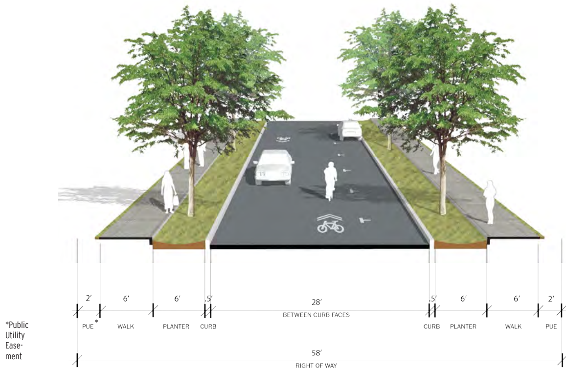
PROPOSED 3ML LOCAL RESIDENTIAL STREET CROSS-SECTION
