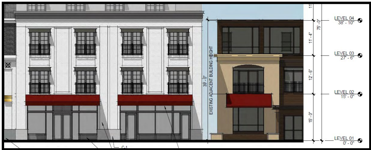
Sheet A3.01 showing the Kaos building adjacent to the proposed three story elevation of the Gwendolyn Hotel that will be property tight on the northeastern corner of the intersection of Ford Street and Third Street.
