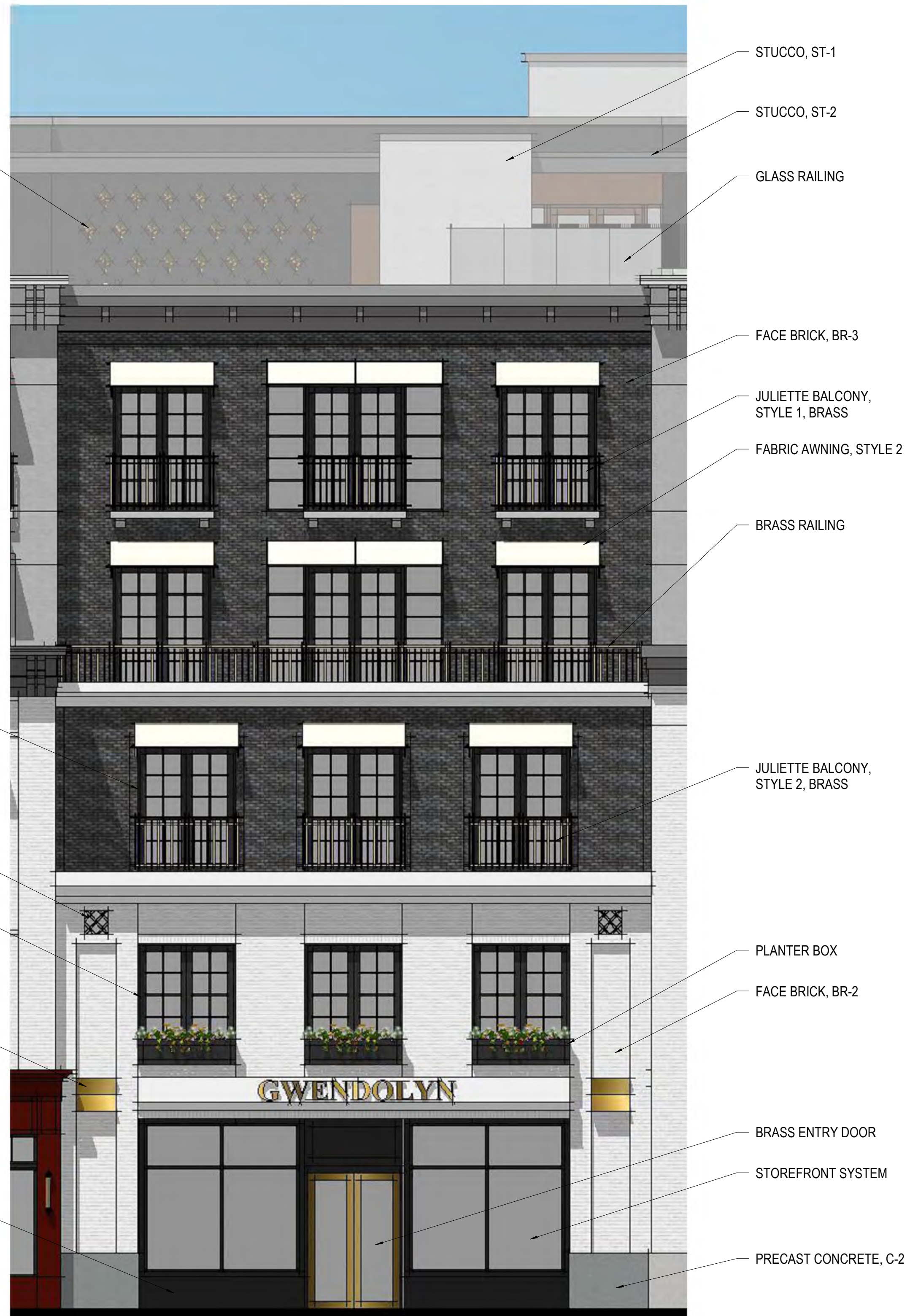
ENLARGED PARTIAL ELEVATION - 3RD STREET
