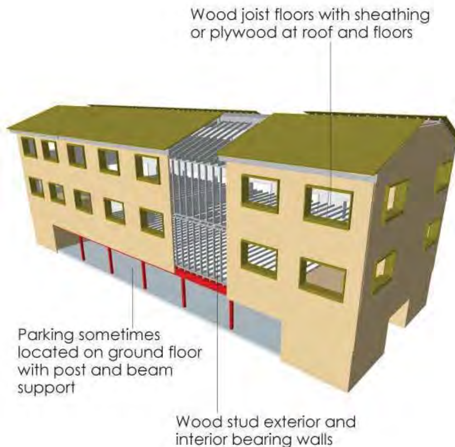
Figure 6.1-1: Building Type W1A: Multistory Multi-Unit Residential Woodframes
