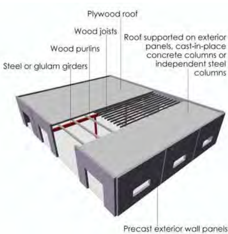
Figure 16.1-1: Building Type PC1: Tilt-Up Concrete Shear Walls
