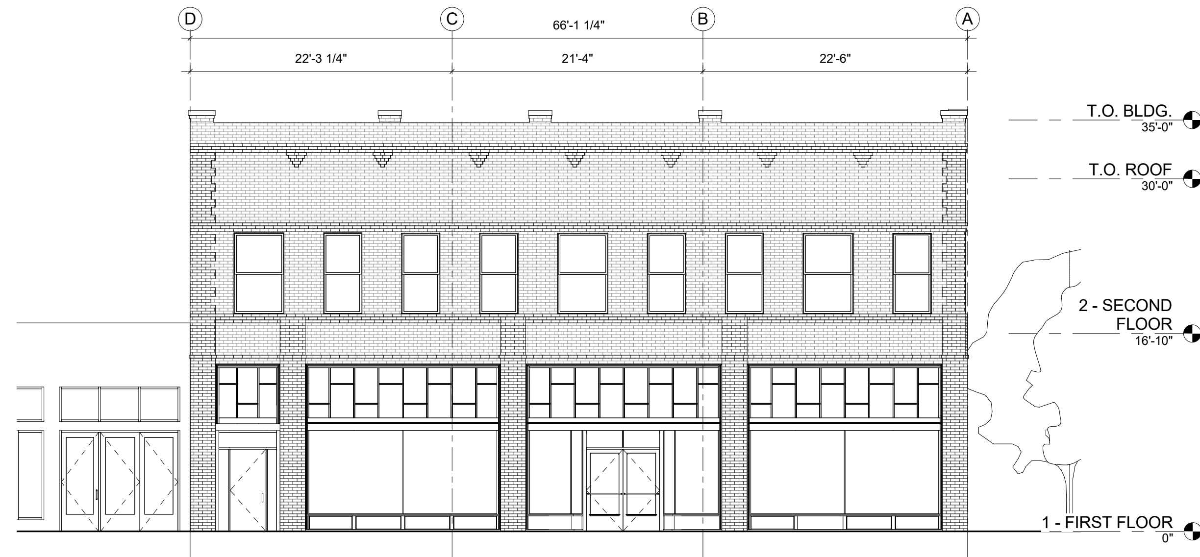
1 NORTH ELEVATION - EXISTING 1/8" = 1'-0"
