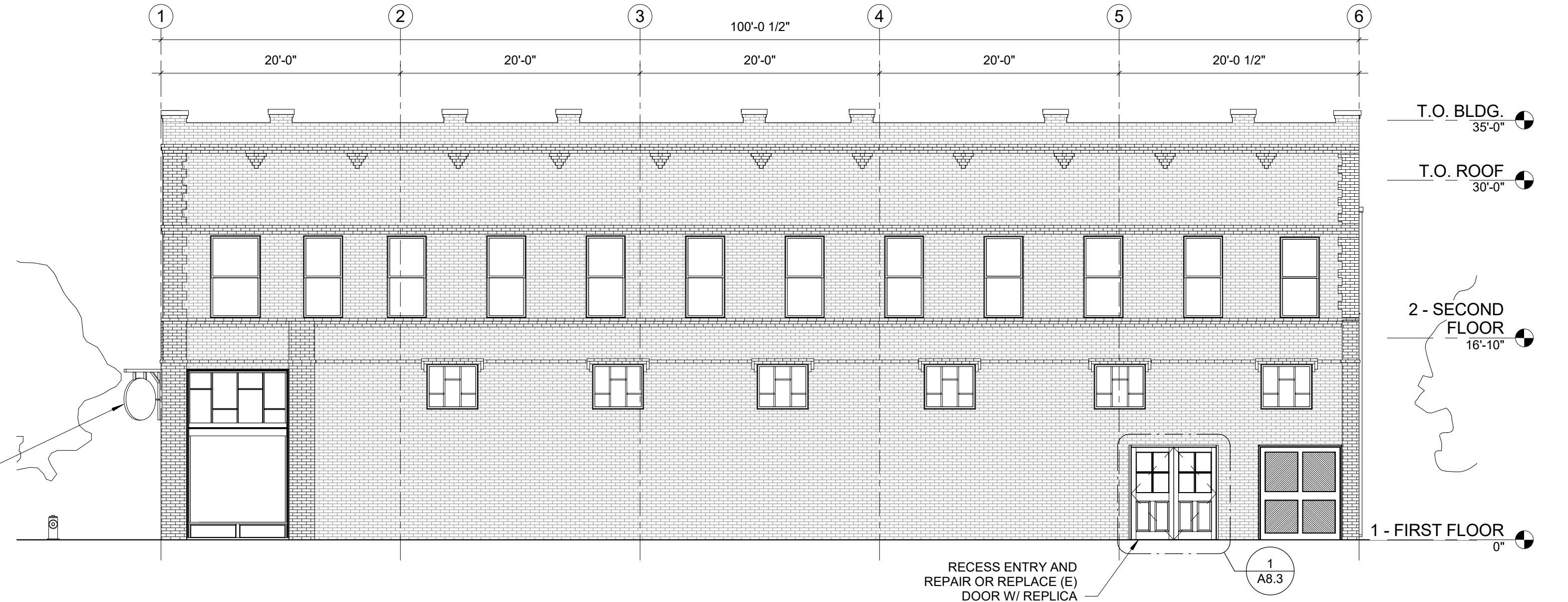
4 WEST ELEVATION - PROPOSED 1/8" = 1'-0"
