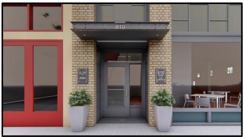
On the west façade, the applicant is proposing to further recess the existing double doors to allow for those doors to open without projecting into the public right-of-way and pedestrian pathway. These doors also need to be changed from in-swinging to out-swinging in order to provide for egress from the ground floor per the building code, and the additional recessed entry will allow for that to occur within the property line.
