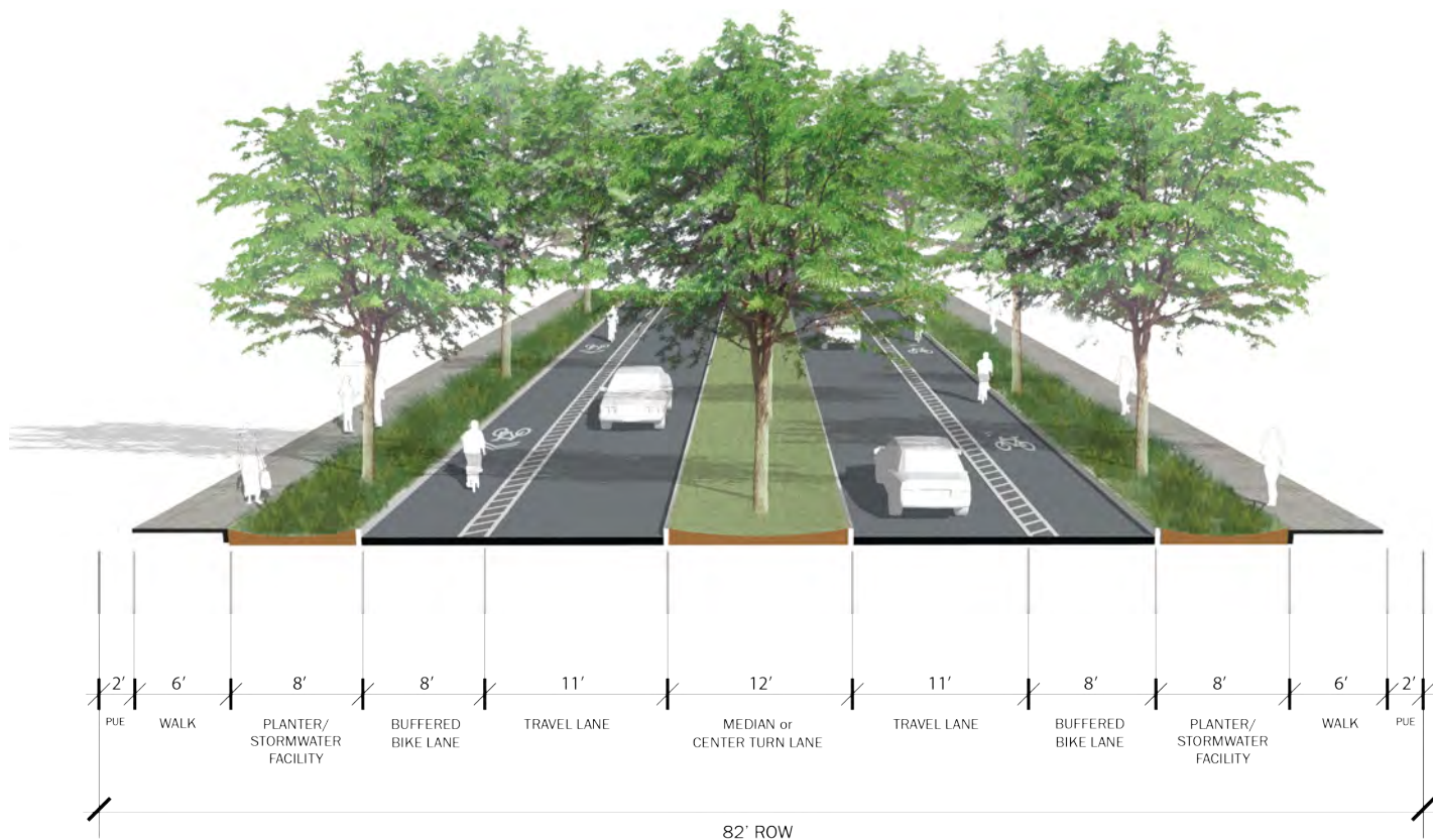
PROPOSED 3ML MAJOR COLLECTOR STREET CROSS-SECTION
