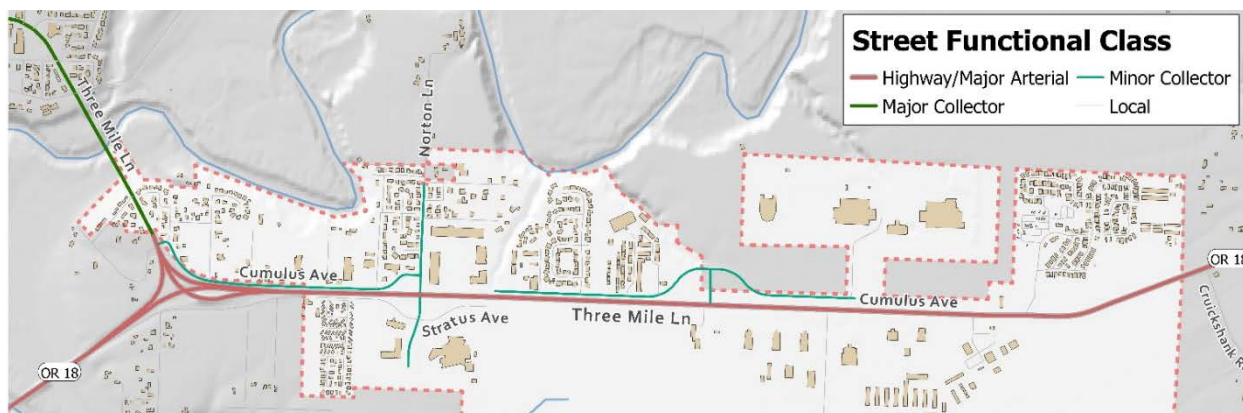
Figure 4. Street Network Functional Classification
