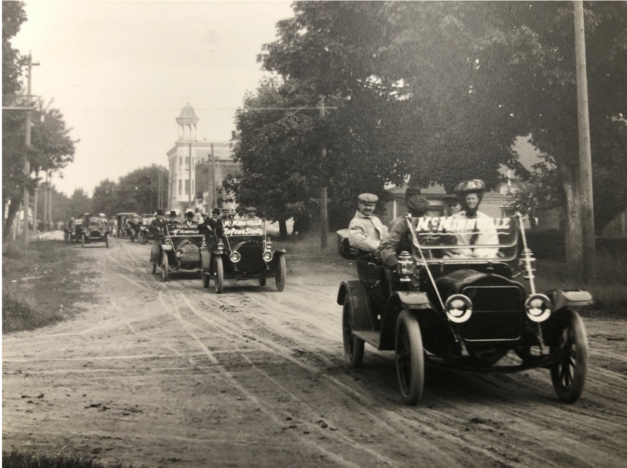
Figure 5, Auto parade at McMinnville during a campaign for paved streets. Ca. 1910. The leading car in figure 5 appears to be a Ford. The three cars behind the Ford that can be identified are Overland touring cars. Note that all four cars are equipped with right-hand steering. OHS
