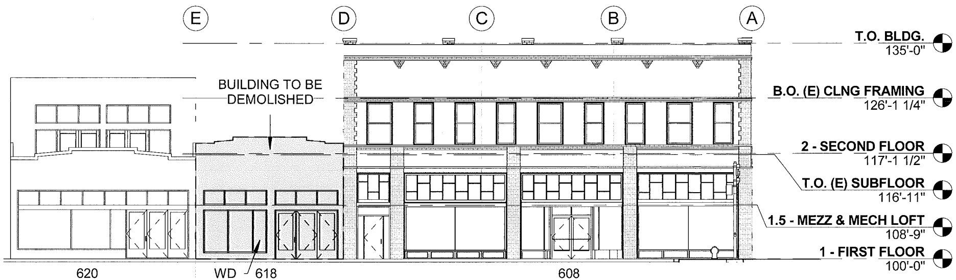
1 EXISTING NORTH ELEVATION 1/16" = 1'-0"
