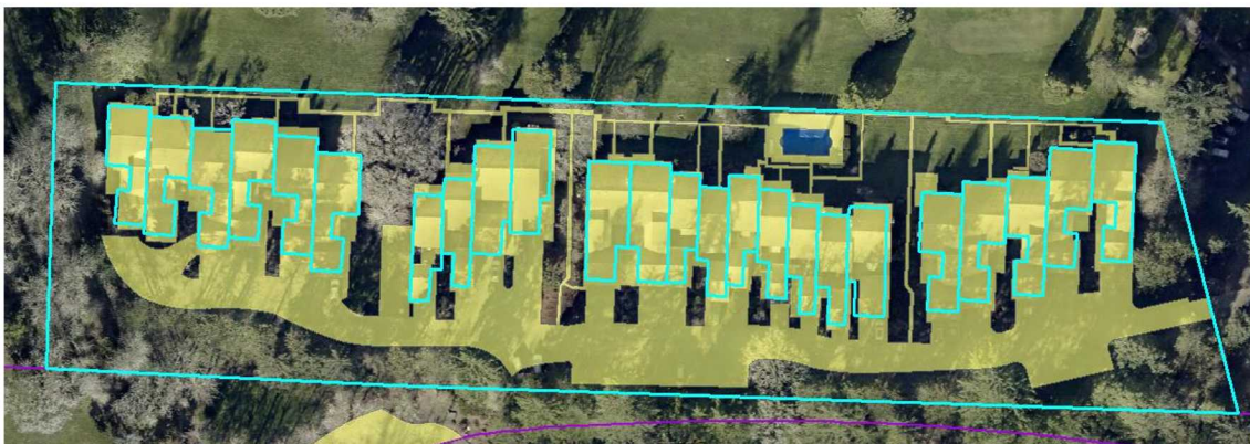
Figure 1. Example of SFA community Impervious Area Digitization (figures not at the same scale)
