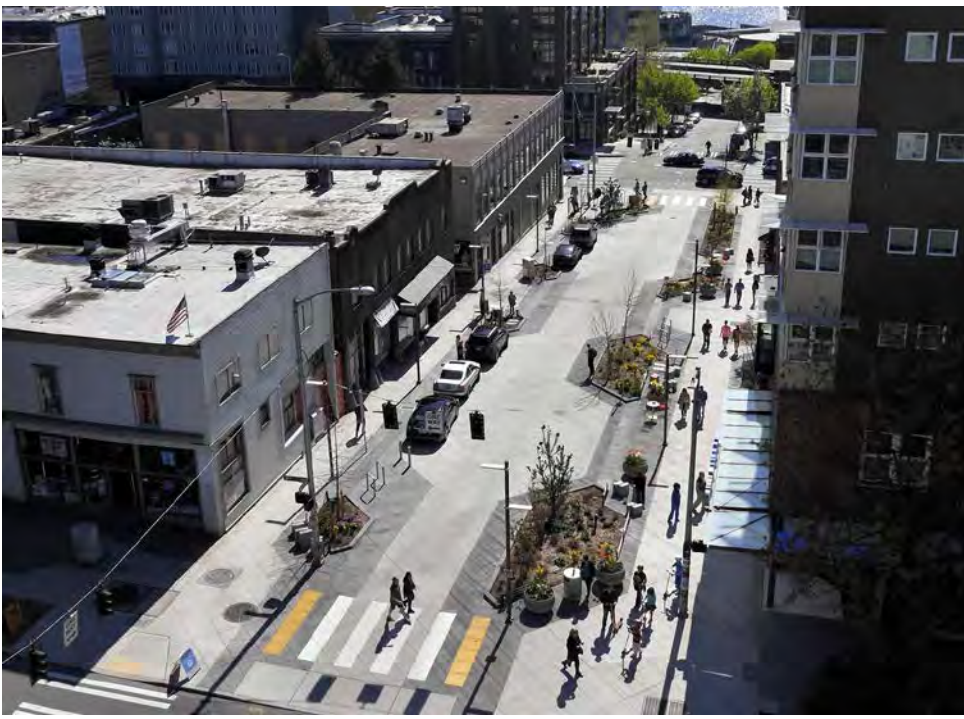
Chicane calms traffic, makes outdoor places (Bell St - Seattle)
